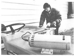
Put 120-volt, AC power for your tools where you want it with this rotary inverter. The inverter plugs into the I-5 tractor's 36 volts DC through the accessory outlet and puts out up to 120 volts AC. High starting capacity for induction motors and up to 1000 watts continuous output.
