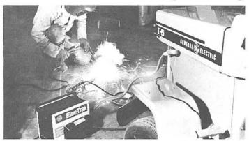
A 180-amp DC arc welder is available for the I-5 Elec-Trak® industrial system. The welder plugs into the tractor for power and three heat ranges allow welding up to one-half inch steel. A welder kit, including helmet, gloves and welding rods is available (AP92).
