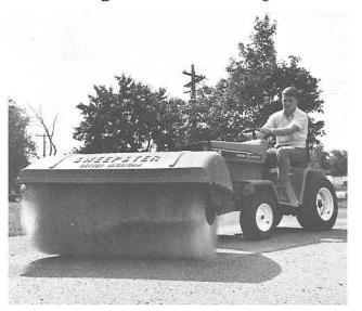
A powerful four-foot wide rotary broom sweeps away debris, including up to 8 inches of snow. A DC motor starts long-wear polypropylene bristles spinning at the touch of a dashboard power take-off switch. Another switch adjusts sweeping pressure or completely lifts the broom with the I-5 electric front implement lift. The broom has three angles of attack. Like all attachments, it detaches in minutes, freeing the I-5 for other duties.
