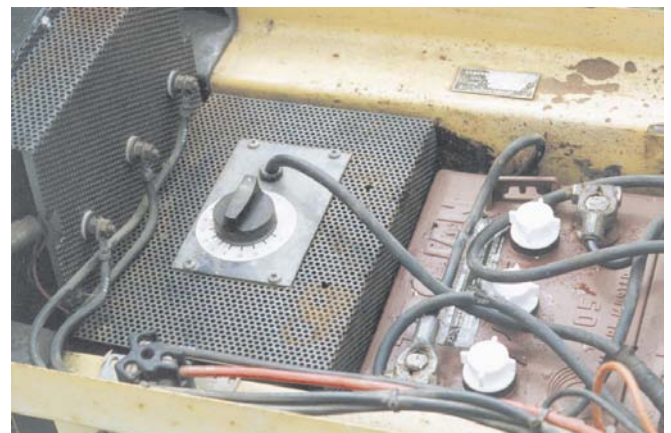
Below: The timer control knob is clearly visible on the E20 charger. The PTO socket is at lower left.
