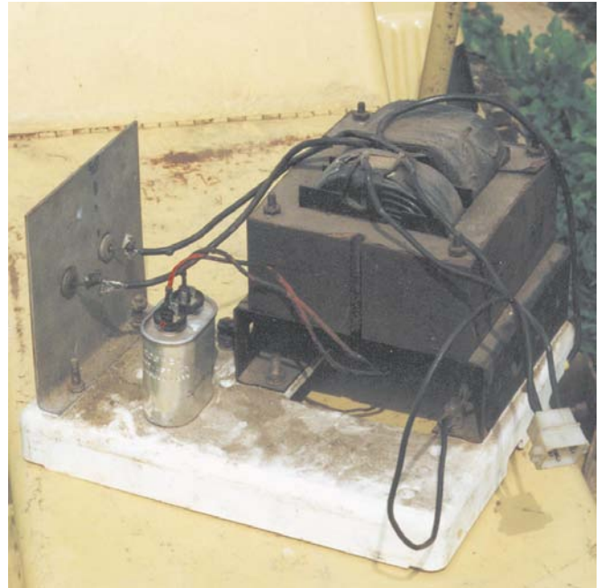
Above: The E20 charger removed from the tractor, showing the heat sink with two diodes, capacitor, and transformer.
