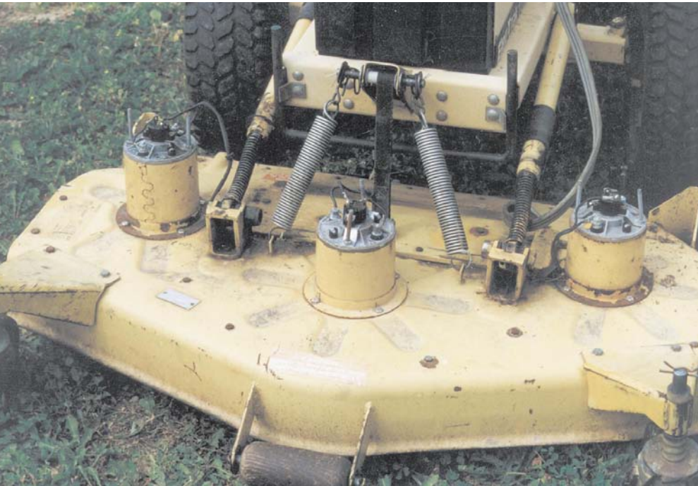
Above: The three motors on the out-front mower deck of an E20.
