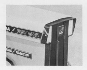
Headlights provide plenty of illumination for night mowing or other tasks. Console controls are lighted by a dashlight.
