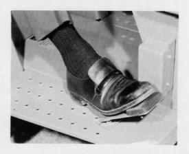
A foot pedal accelerator provides speed control of both forward and reverse motion. The speed of the tractor increases through seven speeds forward or three speeds in reverse as pressure is applied to the foot pedal.
