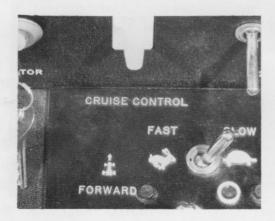
Cruise Control is another exclusive for the EGT-200 and consists of the white push button (upper left) and toggle switch (lower right). Cruise Control locks the tractor into the most efficient operating speed, and may be cancelled either manually or automatically by tripping any one of the tractor safety devices (seat switch, brake switch, etc.)
