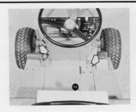
The operating platform is shown in the picture above. All controls, including the foot pedal accelerator (right) and brake pedal (left) are conveniently located and easily accessible to the operator.
