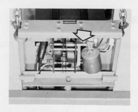
An Electric Lift is standard equipment on the EGT-200. It provides fingertip control of both mid mount and front mount attachments.
