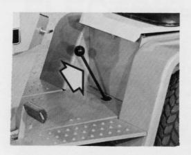
The range selector (shown by arrow) provides a selection of four transaxle gear ranges. To change ranges, the foot pedal accelerator must be in the neutral position (foot off of control). For details of usage of each range, refer to EGT-200 Operator's Manual, page 10.
