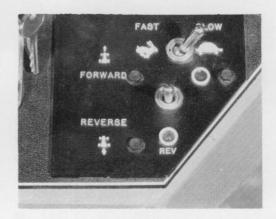
The forward-reverse toggle switch provides a smooth instant change between forward and reverse tractor motion. The red safety pilot light (lower right) remains on at any time the tractor is in reverse.
