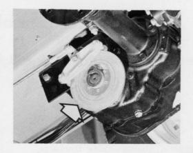
When the brake pedal is depressed this disk brake goes into action to provide safe sure stops. If the pedal is fully depressed, a brake switch (not shown) provides additional safety by disconnecting power to the tractor drive motor.
