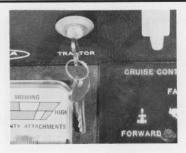
Security and safety are provided by the key switch, which is conveniently located on the tractor console. This switch, when turned clockwise to the 'on' position releases the power from the Power Pack and readies the tractor, attachments, or accessories for instant operation.
