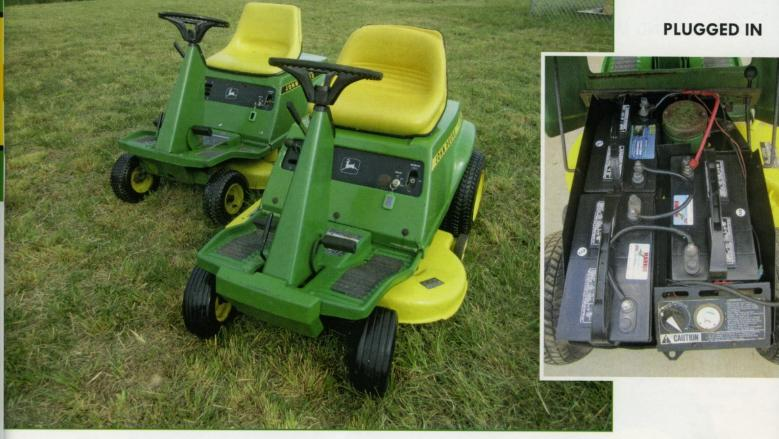
simple resisters to control speed. Want to slow down? Activate a resistor to reduce the amount of electricity going to the motor. Want to speed up? Bypass all the multiple resistors, and let the full current of the batteries reach the traction mower. With a little mechanical knowledge, you can have one restored in no time.
