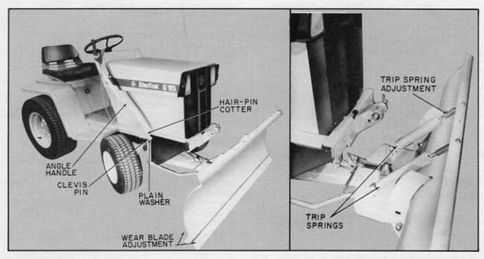
Implement Mounting Bracket, AP 56, must be used to attach the Snow/Dozer Blade to the ELEC-TRAK garden tractor.
