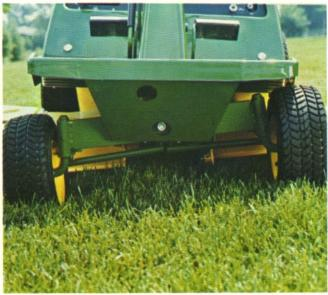
The oscillating front axle helps keep the Electric 90 level when it is operated on uneven ground. Excellent stability is provided by a low center of gravity, uniform distribution of weight, and high-flotation tires.
