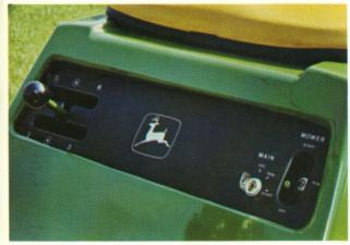
Controls are located on a panel beneath the seat. The gearshift controls ground speed; there are three forward and one reverse speeds. A key switch starts the traction motor and a toggle switch starts the mower. As a safety measure, the traction motor cannot be started unless the clutch is depressed. And if the key is turned off while the mower is running, the mower toggle switch must be recycled before the mower can be restarted.
