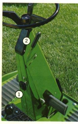
Mower cutting height (Figure 1) adjusts to any distance from one to four inches above the ground. Mower is raised and lowered easily with the lift lever (Figure 2). When the mower is lowered it automatically returns to the preset position. The two-bladed mower is designed for non-scalp mowing. It produces an even discharge of clippings.
