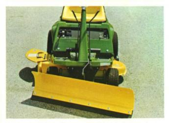
This handy, 38-inch, front-mounted blade is designed for light snow removal. It angles to the right and left of center, raises or lowers easily, and is attached or removed quickly without tools. The rubber squeegee on the blade protects the unit from damage, protects the operator and prevents marring the driveway or sidewalk. A belt drive protects the drive train from damage should the Rider strike an unyielding object.
