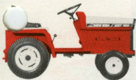
EGT-120 (14-hp Class) mows 42" swath with front-mounted mower.
