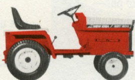
EGT-200 (18-hp Class) Electric Garden Tractor has 42" front- or mid-mounted mower.
