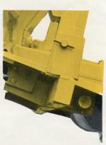
Illustration shows CROSS MEMBER - this allows for instant, simple mounting or dismounting of the rugged formed frame to the tractor.
