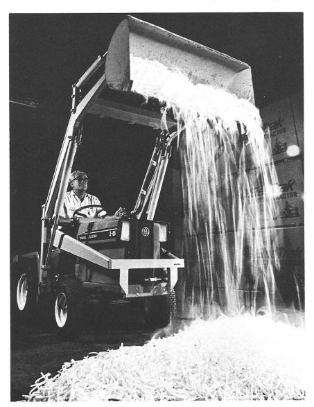
Loading and transporting bulk material no longer means noisy, smoking bucket loaders. This unique 500-pound capacity loader for the Elec-Trak tractor operates on electrically powered hydraulics. The self-leveling bucket gets its lift from double-acting cylinders. Two levers near the dashboard control the bucket lift. Plenty of down pressure is available. Sold with weight box.
